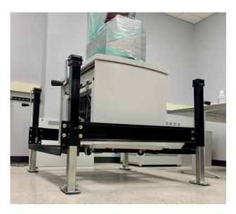
3. The third step is to place the platform under the microscope and then level the vibration isolation platform to spec
