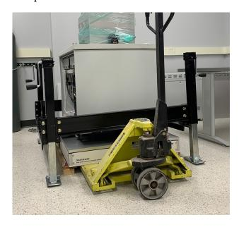
4. Next, VEC will carefully lower the microscope onto the platform and then dismantle the custom microscope lift.
